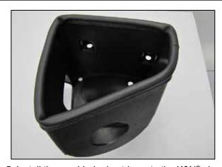
5. Install the provided edge trim onto the K&N® air filter housing as shown.
